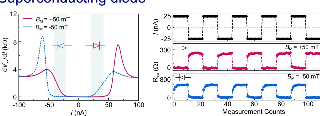
The non-reciprocal transport caused by the current-field coupling enables us to realize a programmable, zero-field superconducting diode. By applying a DC current in opposite directions, we can measure a rectifying behaviour in the sample, which can be switched by previously magnetizing the device at positive or negative low fields.
