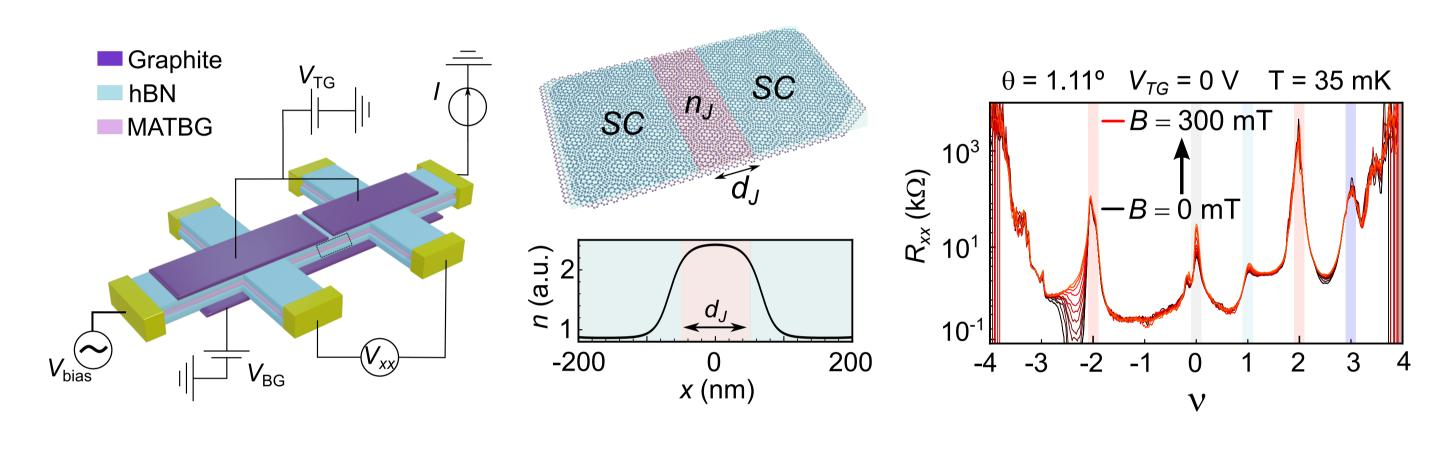
The gate-tunability of MATBG and our three-gated geometry allows to create junctions made of the same material, thus with ultra-clean interfaces. This enables us to probe the correlated states of our device in a narrow region  $d_J \sim 100$  nm with a JJ.
