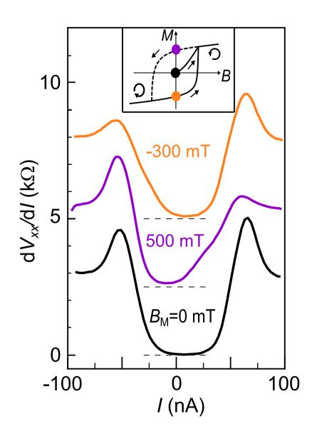
By pre-magnetizing the sample at  $\sim \pm 300$  mT, the dV/dI curve becomes asymmetric at zero field. The current direction is thus affected by the field.
