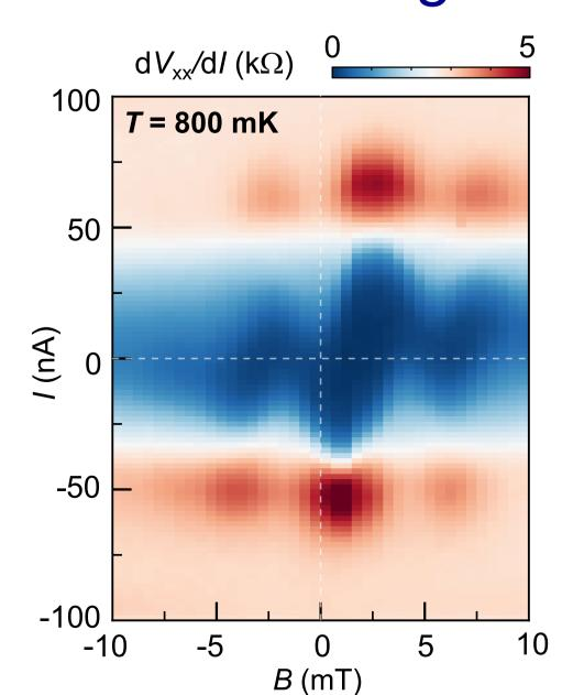
Non-symmetric Fraunhofer pattern with respect to the current and field. Time-reversal symmetry is broken and therefore the relation  $I_c^+(B^+) = |I_c^-(B^+)|$  is not satisfied.
