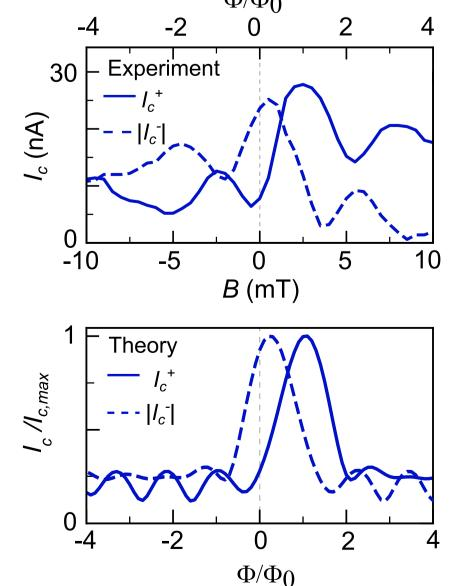
Our data is reproduced by simulations of a JJ with an orbital magnetic state with Chern number C=-2 set as the weak link. The current induces orbital magnetism.
